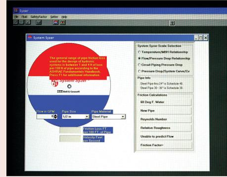
Scale #2 can also be very helpful when you are out in some boiler room trying to select a new pump. If all of the tags from the boiler and original pump are missing, you can use the existing main hot water pipe as a guide. Based upon its size, you can look on Scale #2 and determine the MAXIMUM flow that particular pipe can handle. It at least gives you a basis from which to build your theory.
