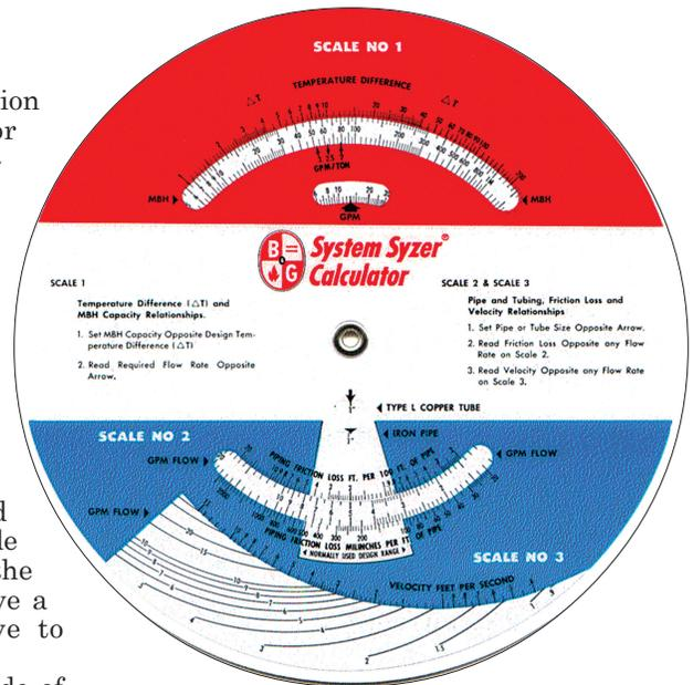
show them how they can select smaller flow rates (GPM) by simply increasing the system's allowable temperature drop. Traditionally in this industry we design around a magical number of 20°F temperature drop. By simply increasing this temperature drop to 40°F, you will have successfully cut your required flow rate in half. It's all right there on scale #1!
