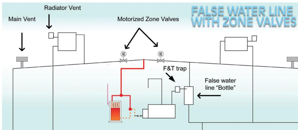
portion of the wet returns, which would create incredible banging and clanging noises. The key to a successful false water line installation is to mount the bottle or large Float & Thermostatic trap (F&T) at the water line height of the original boiler. That way, you are assured that all of the original piping that was wet remains wet and everything above the old boiler's water line stays dry. (See Figure 2)
