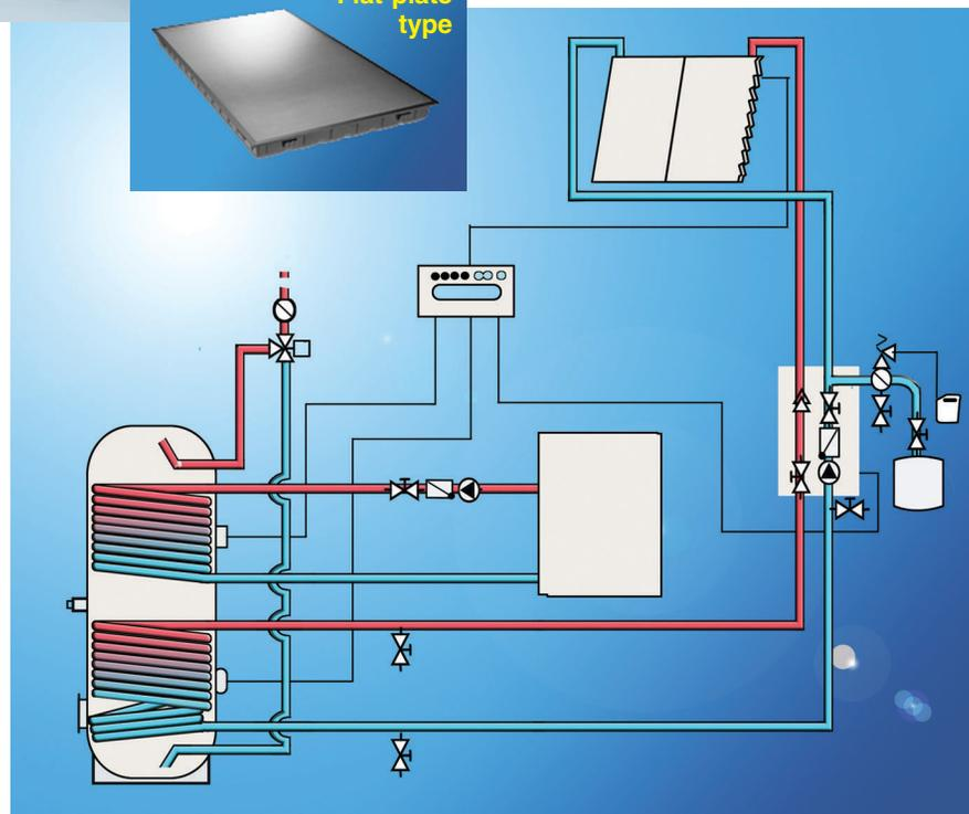
classification. I would like to focus on systems that are considered active (use of circulators to move liquid through the solar collector) and that are designed to collect solar energy for heating buildings and/or domestic water.
